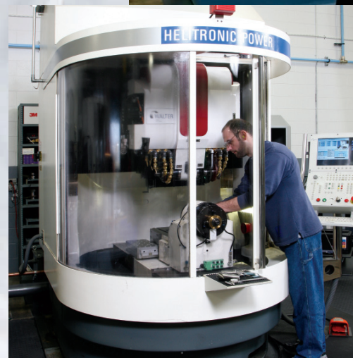
The Walters power CNC tool grinder probes a tool before grinding.
